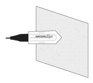
during installation. To limit the effect of water moving vertically through the soil profile, the sensors should be installed so the flat face is perpendicular to the soil surface. For the same reason, if sensors are installed at multiple depths, they should be offset from one another.
