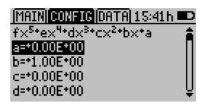
Each coefficient corresponds to a letter in the polynomial above. Below the polynomial is the value of each coefficient in scientific notation. To edit a coefficient, press **ENTER** when the desired coefficient is highlighted. You will see a screen like the one below.
