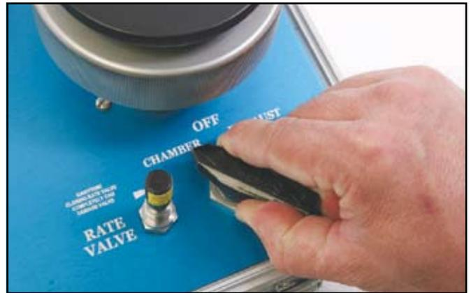
4. Turn the control valve to **EXHAUST** position to release pressure from the chamber. Remove the lid and solid rubber stopper from the inside of lid. You are now ready to take readings.
