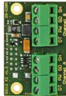
SDI12_X2 Internal Interface for 2 Soil Moisture Probes
