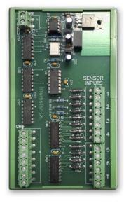
When using an earth grounded reading device OR when using more than one WATERMARK per reading device, the 200SS-V-6 Channel Isolator provides these features:
