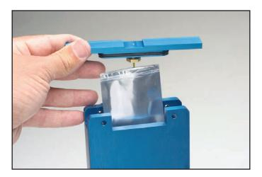
6. Ensure you are wearing eye protection in case sample slips out of chamber. Place foot on footrest, swing eye lens in place and adjust as needed. 7. Begin pumping the chamber by grasping handles and lifting chamber completely to the stop, then pushing down to the stop. Each cycle will increase pressure by about 1/2 Bar or 7 PSI. While pumping on the down stroke, watch sample through eye lens for a film of water to appear. When water appears, stop pumping and record pressure indicated on gauge.
