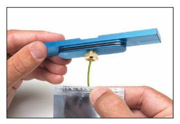
4. Turn Compression Gland Screw clockwise to tighten the gasket around the sample. This depends upon which lid is being used. With the Small Lid, the Compression Gland Screw is made of brass and is on the inside edge of the lid. The Large and Grass lid have an anodized blue Compression Gland Screw that is external.
