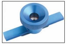
5. Put leaf inside chamber and lock down the lid into chamber. Place Chamber Pins completely through holes so they are in locked position.
