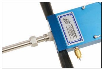
3. If Pressure Relief Valve becomes obstructed with dirt or plant debris, clear this by blowing compressed air in reverse through the valve. Cycle the valve several times while blowing air. This should clear any obstruction.
