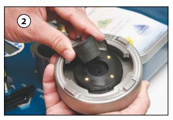
Insert a solid rubber gasket into the lid
