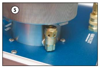
Then turn the lid back so that the cam is not blocking the piston
