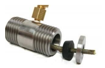
The rubber gaskets slide down the sample and seat inside the chamber.
