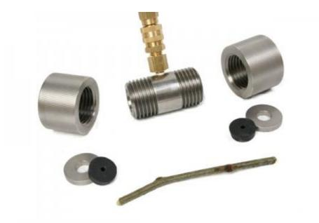
The cavitation chamber feature of this instrument is used to simulate cavitation of xylem vessels in plants under stress. A plant stem, limb or root is introduced into the Cavitation Chamber and a head of water is connected to the sample to measure water conductivity. The chamber is then pressurized to "seed" air into the xylem. It can be used to establish vulnerability curves in plants or to continue <u>research</u> in the area of xylem cavitation.
