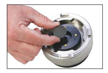
Turn control valve to **CHAMBER** position and pressurize the chamber. Adjust **Rate Valve** until pressure in the chamber increases at the desired rate. ½ Bar per second is a recommended rate of increase. Rate may be changed at any time, even while pressurizing a sample.
