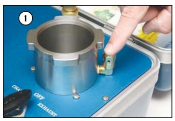
First, use your finger to depress the piston so that it is inside the safety valve
