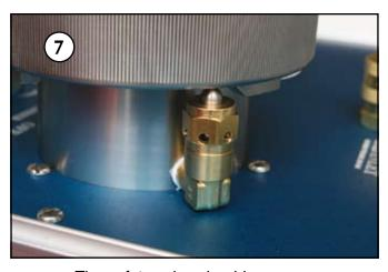
The safety valve should pop open before the pressure reaches 2 bar
