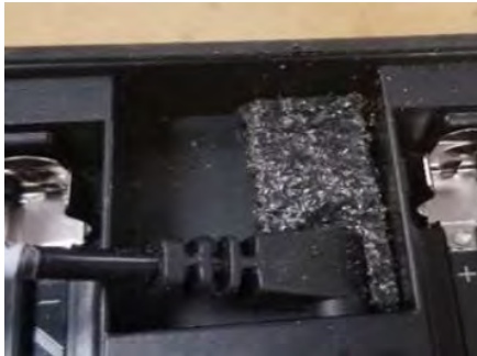
Fig. 2: Foam plug installed
