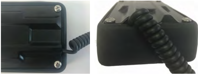
Figure 2. Sensor cable fed through slot
