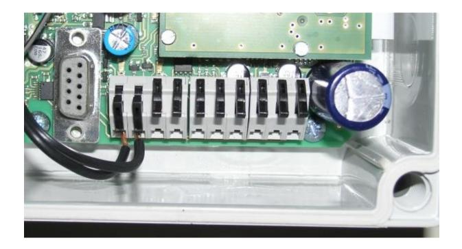
Any digital Sensor can be connected on either digital connection No. 1 or digital connection No. 2 (Picture: One digital Sensor is connected to Port No. 1)
