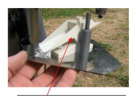
The tipping bucket has to switch back and forth. Clean the mechanism from cobwebs One "tip" is counting 0,2mm of rainfall
