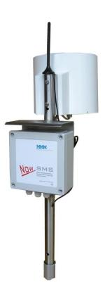
Reset the rain gauge to zero after the final placing in the field, since the tipping bucket has switching back and forth and begins to count during the in-field installation.
