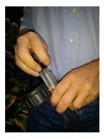
Step 2: fill Tensiometer completely with water
